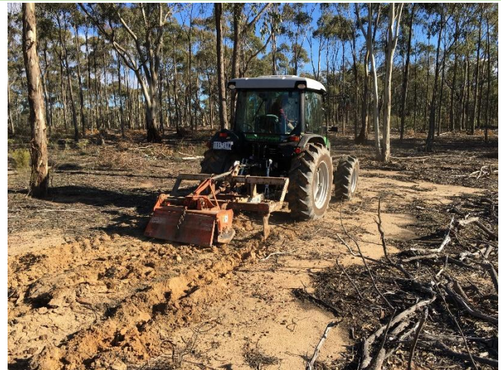
Image 6: Use of tractor to establish keyline (contour) ripping in regrowth forest with degraded ground layer (i.e. striped top soil, exposed compacted subsoil, sparse understorey) typical of Box Ironbark bushland throughout central Victoria.
