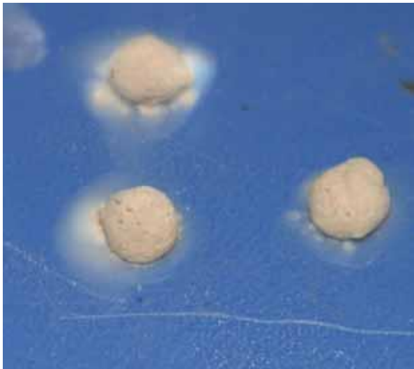
Re-moulded soil: Moderate dispersion at 2 minutes
