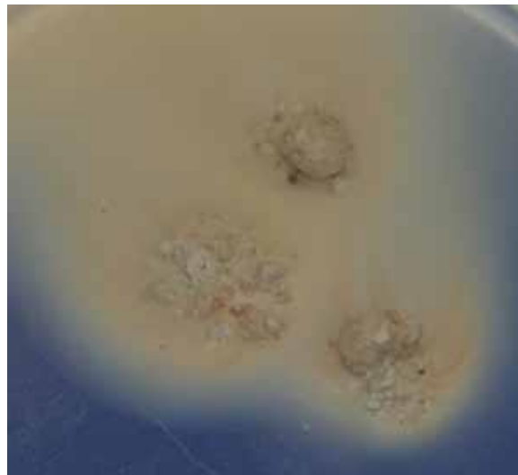
Re-moulded soil: Extensive dispersion at 2 minutes
